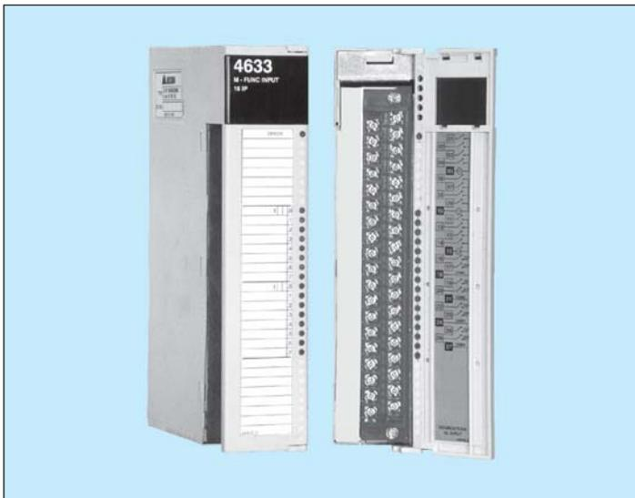
The Multifunction Input module provides mix of inputs with programmable filter time, pulse catch input, interrupt input and counters with programmable 16 bit operational mode. Programmable filter (10ms) and up counter is the default configuration. The alternate configuration can be easily set using DOXMINI+. In such case, the inputs are not available as normal inputs.
