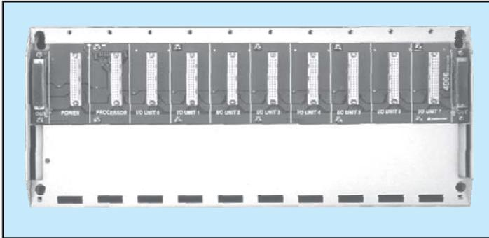
The base plate holds Power Supply, CPU and I/O modules. It is available in varieties to suit I/O and expansion requirement. The base plate is available with or without expansion connector to offer economic solution. Both the base plates are available in 3 I/O, 5 I/O and 8 I/O slots.
