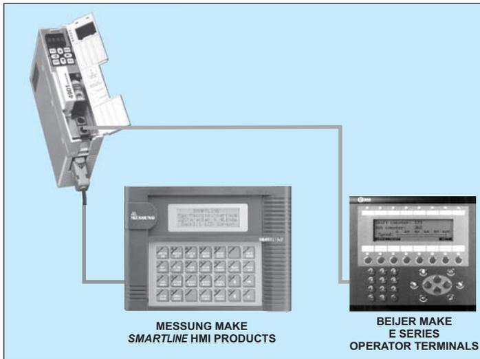
For interfacing one of the HMIs, from SMARTLINE Series Human Machine Interface or Beijer make E-Series Operator Terminals.
