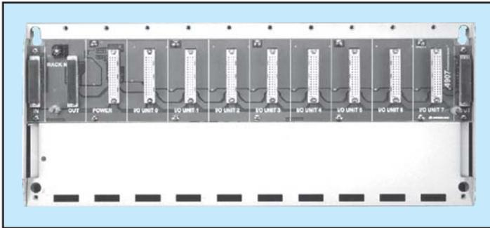
In multi-rack system, the expansion plate can be mounted next to each other or one below other. The expansion plate is available in varieties to suit I/O and power supply requirement. It is available with or without power supply connection facility. Both the expansion plates are available in 3 I/O, 5 I/O and 8 I/O slots.
