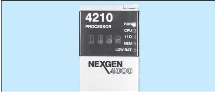
The CPU provides 4 character alphanumeric display. Besides system messages, it can be programmed to show messages related to fault or status in an application.
