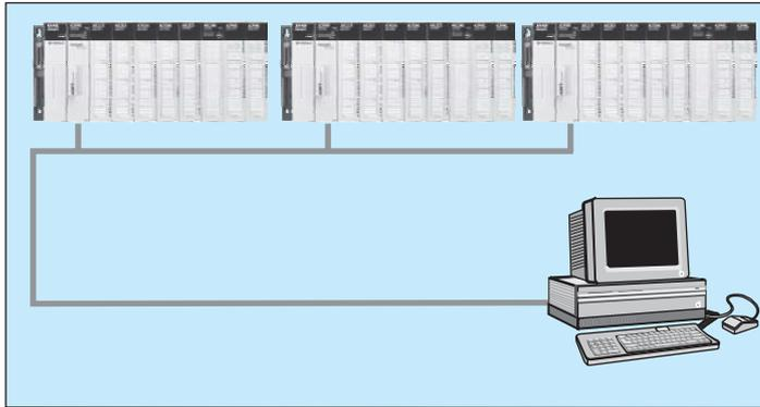
At times, data from multiple PLCs needs to be accessed (for eg. SCADA). In such a case, the third port can be configured as a ASCII port. Now multiple PLCs can be connected in multidrop topology. The hardware interface is RS485. The network topology is single master and multiple slaves. At the most 31 PLCs can be connected.
