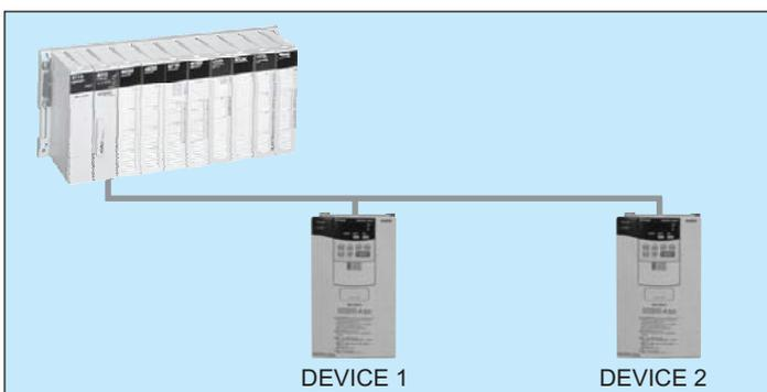
The intelligent peripheral devices like printer, inverter can be interfaced to PLC easily and economically. Only hardware interface details and protocol information is required for interfacing.
