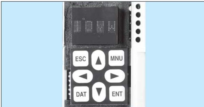
Unique built-in diagnostic tool is provided in the form of 8 keys keyboard and 4-character alphanumeric display. It is useful for
